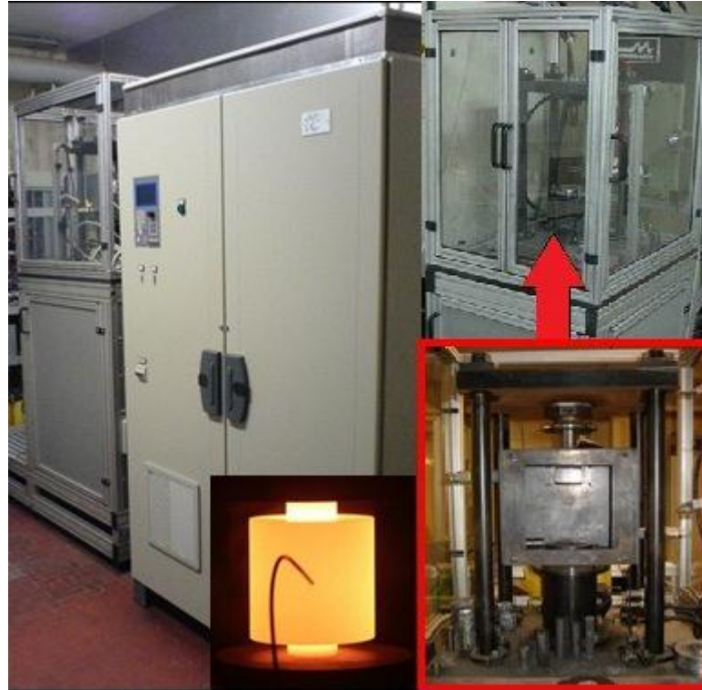
Figure 40 - The PAFES apparatus. In the red panel the sintering chamber.
