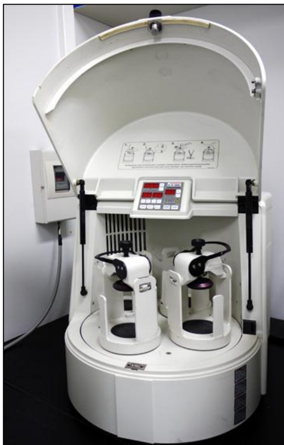
Figure 34 - Planetary milling device
