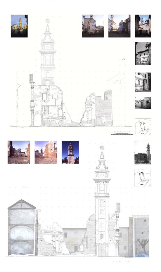
Figure 7. 2D representation of the results: photogrammetric survey, rectified images and photographic documentation (drawing by Paolo Piumatti)
