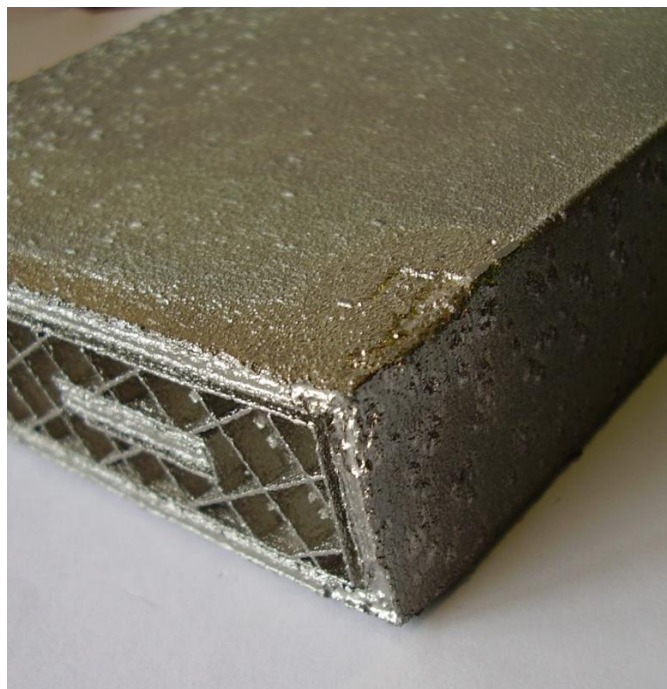
Figure 1: EBM sintered workpiece, as supplied
