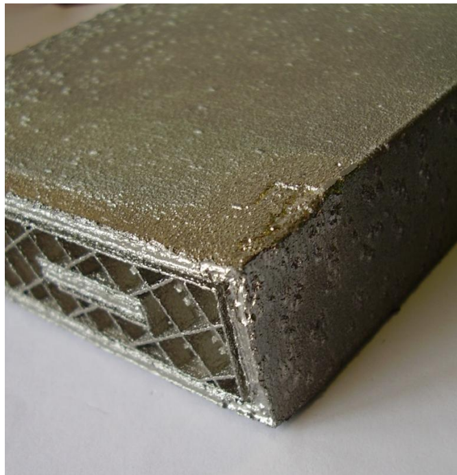
Figure 1: EBM sintered workpiece, as supplied.
