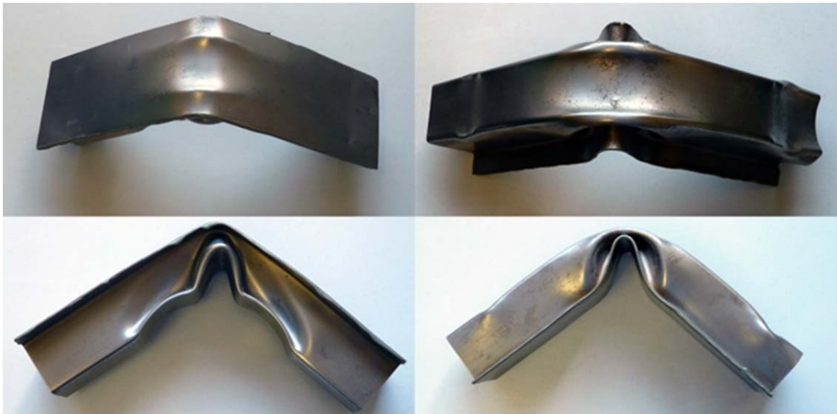
Figure 12: metal specimens joined by adhesive after the test; on the left plate on the top, on the right plate in bottom position
