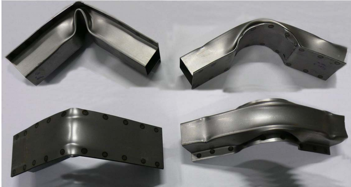
Figure 14: metal specimens joined by spot welding after the test; on the left plate on the top, on the right plate in bottom position
