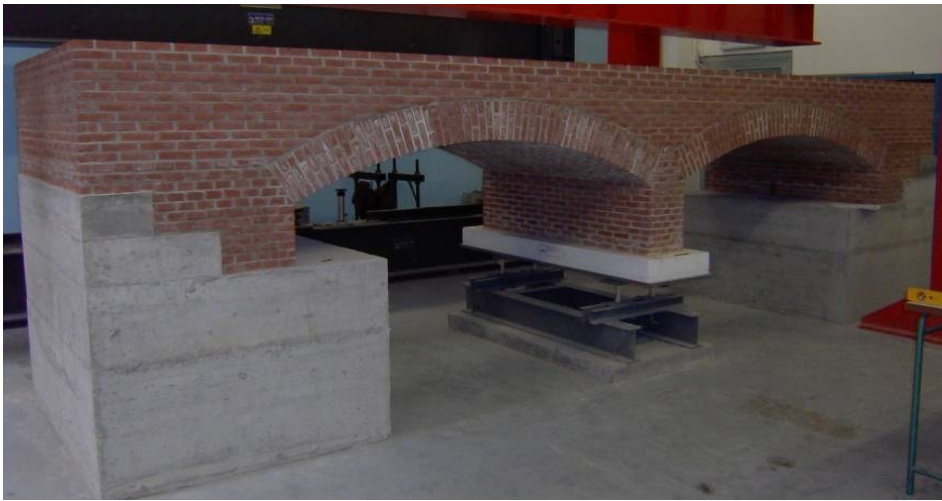
Figure 1. The scaled masonry bridge: notice the settlement application device under the central pier
