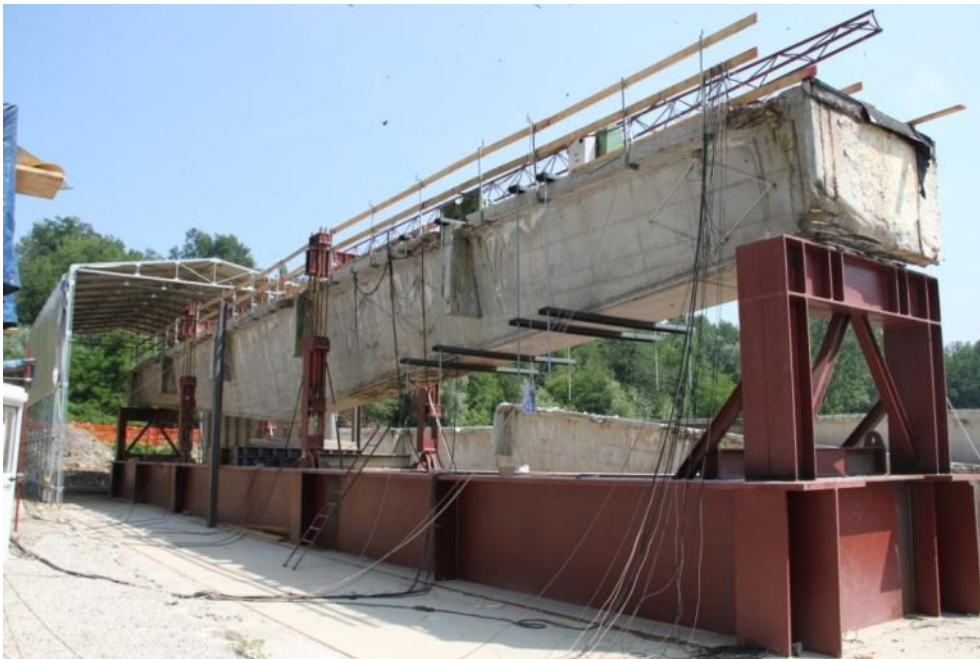
Figure 21 Beam B04 placed on the test bench
