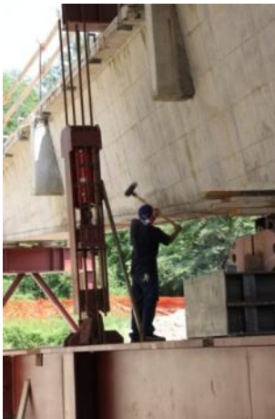
Figure 7 A phase of execution of the impact test and an example of the acquired signal
