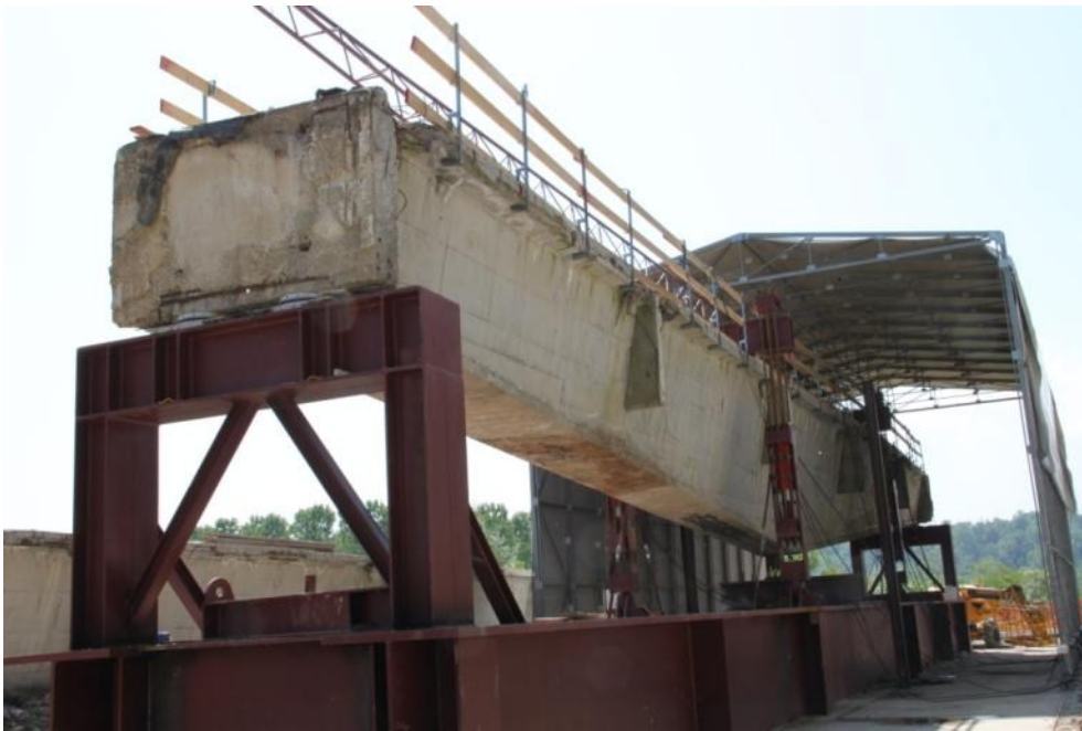
Figure 11 Beam B02 placed on the test bench
