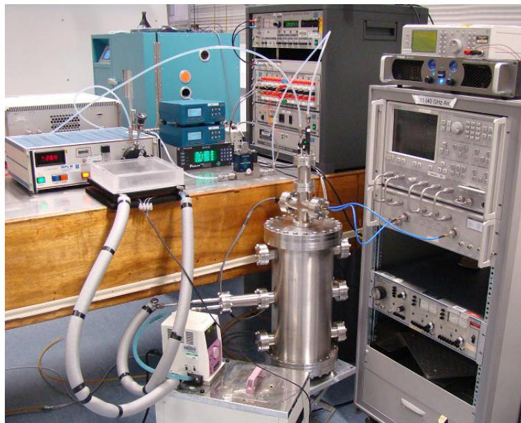
Figure 5.2: Experimental apparatus realised at the Acoustic Thermometry laboratory of NPL for condensation tests.
