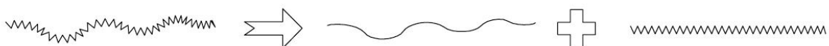
Figure 1.12 - Example of filtration operation used to separate the form error components of a straightness profile [14].
