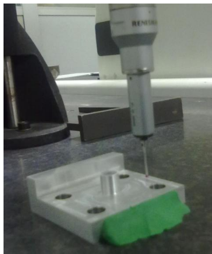
Figure 6.1 – The case study's flatness feature, on the measurement bench of CMM (model: Dea Iota 0101), for the tolerance verification. Tolerances are reported in Figure 3.1.
