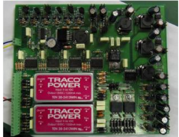
Figure 17. Electric power electronic board.
