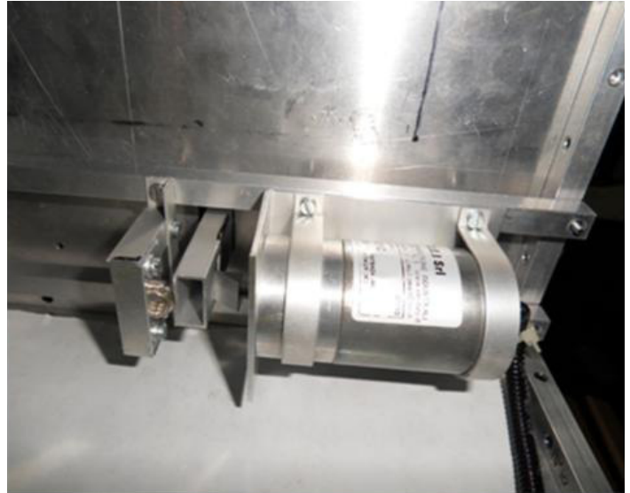
Figure 24. Undocking/separation subsystem: the latch.
