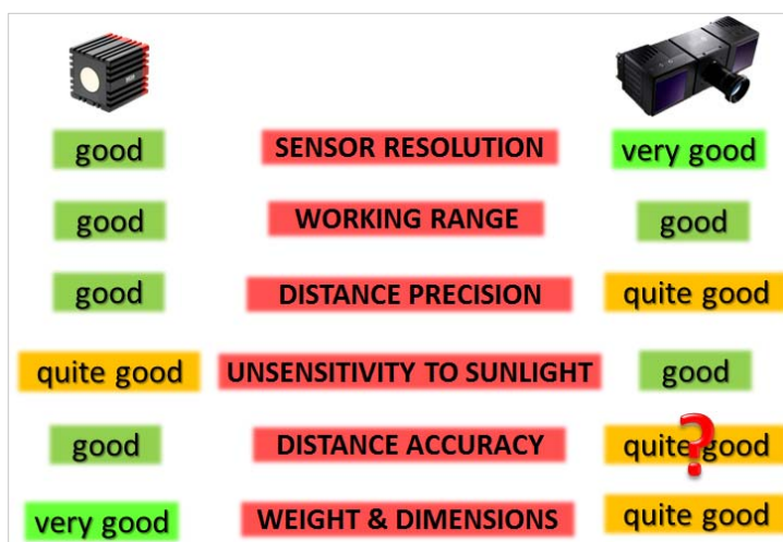
Figure 13. Comparison between SR-4000 camera (left) and CamCube3.0 camera (right) based on the performed tests.
