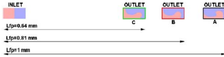
Fig. 14 Interface deformation at the outlet section of (a) the fixed-curvature segment, (b) the clothoid segment with same length as geometry A and (c) the clothoid segment with initial curvature as curvature of
