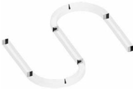
Fig. 15 A meander micromixer unit, made of two fixed-curvature segments operating at Re=10 . Two coloured stream are inserted at the inlet section (left side) and in consequence of secondary flows undergo an increment of contact area which reduces during the reversal of curvature showing kinematic reversibility
