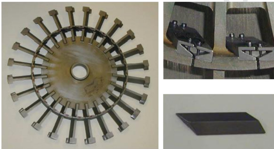
Fig. 5. Test article: the blisk, the blade inserts and the damper.
