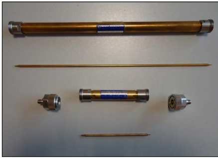
Figure 1: The two coaxial airlines used for the measurements of the S-parameters
