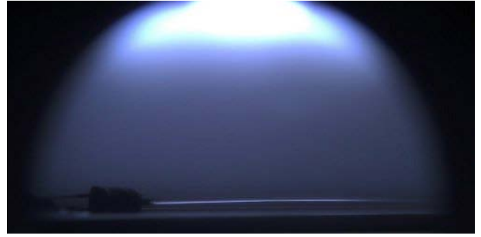
Fig. 2. The fiber in the plasma reactor during the coating deposition.
