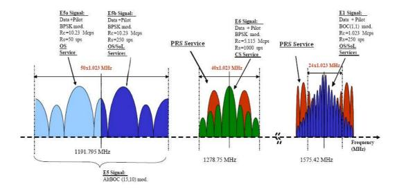
Figure 1.5: Galileo signals and mapping to services [4]
