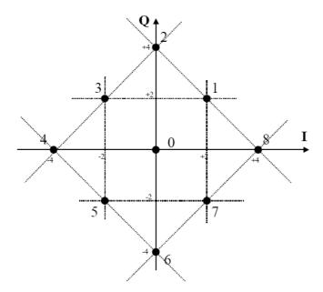
Figure 2.15: Scattered plots for standard AltBOC modulation [9]
