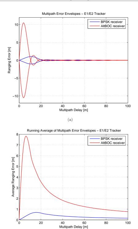
Figure 6.25: Multipath performances with the Early1/Early2 tracking technique: multipath error envelopes (a) and running average of multipath error envelopes (b), for the two receiver architectures
