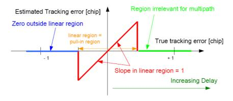
Figure 6.28: Optimum linear S-Curve for the shaping technique [46]
