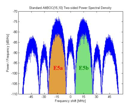
Figure 2.14: Standard AltBOC(15,10) signal spectrum
