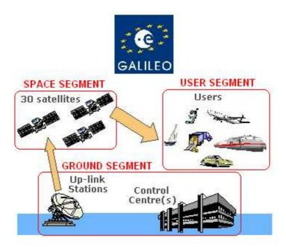
Figure 1.2: Architecture of the GALILEO system
