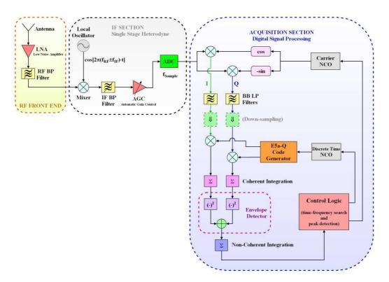
Figure 5.13: Block diagram of the single band receiver architecture, with the SSB (E5a sideband) acquisition section
