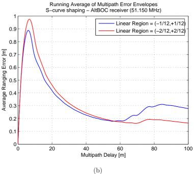
Figure 6.41: Comparison of multipath performances with the S-curve shaping technique, varying the linear region: multipath error envelopes (a) and running average of multipath error envelopes (b) with the AltBOC receiver with a bandwidth of 51.150 MHz, using a linear region of  $\pm 1/12$  chip (scenario 6) and a linear region of  $\pm 2/12$  chip (scenario 7)
