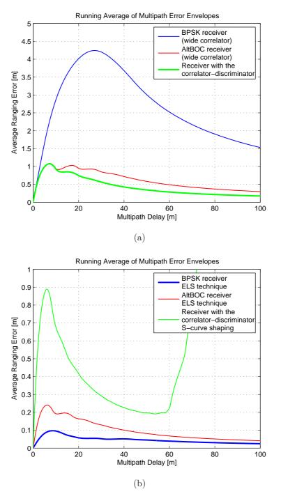
Figure 6.61: Comparison of multipath performances obtained with the three receiver architectures: the BPSK receiver (30 MHz), the Alt-BOC receiver (51.150 MHz) and the receiver with the correlator-discriminator (51.150 MHz). Comparison of running average of multipath error envelopes for the three receivers without multipath mitigation (a), and multipath performances obtained with the best multipath mitigation technique for each receiver (b)
