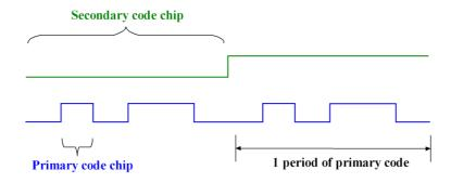
Figure 2.5: Illustration of the tiered code structure
