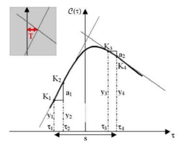
Figure 6.22: General concept of the Early/Late Slope technique: computation of a pseudorange correction T by analyzing the slopes on both sides of the correlation function
