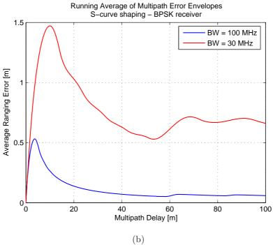
Figure 6.35: Multipath performances with the S-curve shaping technique, for the BPSK receiver with finite bandwidth signals: multipath error envelopes (a) and running average of multipath error envelopes (b), for a bandwidth of 100 MHz (scenario 3) and 30 MHz (scenario 4)
