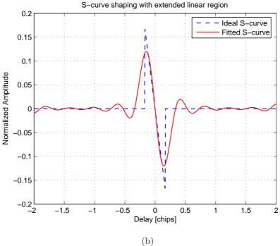
Figure 6.39: Correlator diagram and obtained S-curve for the shaping technique with extended linear region (scenario 7): correlator positions and weights (a) and obtained S-curves (b) with the AltBOC receiver, using a bandwidth of 51.150 MHz and a linear region of  $\pm 2/12$  chip
