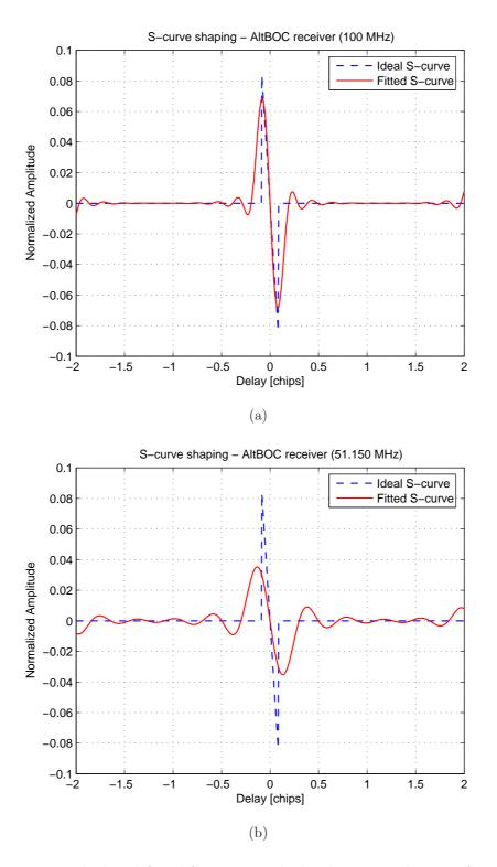
Figure 6.36: Ideal and fitted S-curves with the shaping technique, for the Alt-BOC receiver with finite bandwidth signals: obtained S-curves in scenario 5 (a) and in scenario 6 (b)
