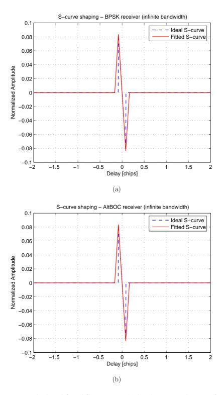
Figure 6.32: Ideal and fitted S-curves with the shaping technique, for infinite bandwidth receivers: obtained S-curves with the BPSK receiver in scenario 1 (a) and with the AltBOC receiver in scenario 2 (b)
