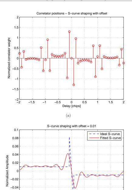
Figure 6.42: Correlator diagram and obtained S-curve for the shaping technique with offset (scenario 8): correlator positions and weights (a) and obtained S-curves (b) with the AltBOC receiver, using a bandwidth of 51.150 MHz and an offset of 0.01 (normalized value)
