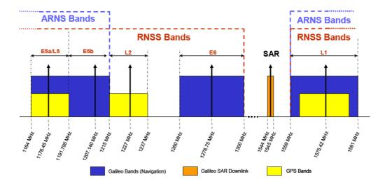
Figure 1.4: Galileo frequency plan [4]
