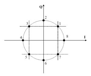
Figure 2.21: 8-PSK phase-state diagram of E5 AltBOC signal [9]
