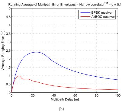
Figure 6.18: Multipath performances with the narrow correlator  $^{\text{TM}}$ , using a spacing of d=0.1 chip: multipath error envelopes (a) and running average of multipath error envelopes (b), for the two receiver architectures
