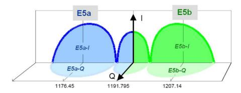
Figure 2.20: Spectral scheme for Galileo E5 band
