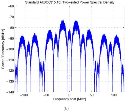
Figure 3.5: Comparison between the E5 AltBOC(15,10) signal spectrum (a) and the Standard AltBOC(15,10) signal spectrum(b)
