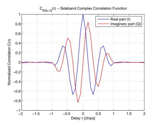
Figure 3.7: Sideband complex correlation function  $C_{E5b\text{-}Q}(\tau)$ , for the pilot channel of the E5b band
