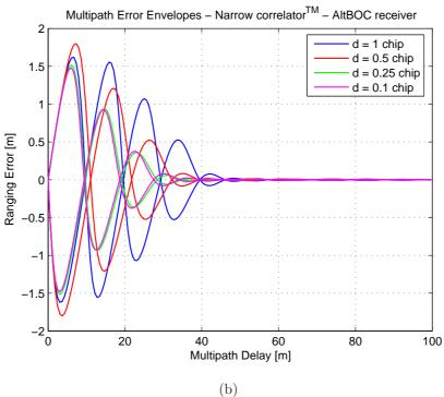
Figure 6.17: Multipath error envelopes for a narrow correlator  $^{\rm TM}$  using different correlator spacings, for the BPSK receiver (a) and the AltBOC receiver (b)
