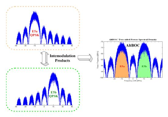
Figure 3.4: Illustration of AltBOC signal spectrum, like a multiplexing of two separate QPSK modulations
