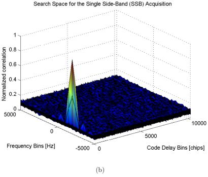
Figure 5.19: Example of SSB acquisition performed with the E5a-Q pilot code, simulated with a coherent dual band receiver, with infinite bandwidth and in presence of noise (SNR = -10 dB, C/N<sub>0</sub> = 60 dB-Hz at the input of the acquisition section): resulting search spaces with 1 single non-coherent accumulation (a) and with 10 non-coherent accumulations (b)
