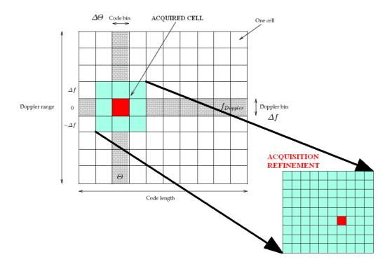
Figure 5.9: Progressive acquisition scheme
