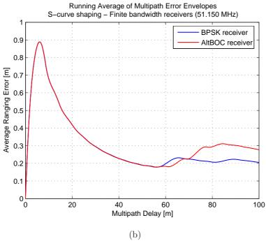
Figure 6.46: Comparison of multipath performances with the S-curve shaping technique, for the two receiver architectures using the same limited bandwidth (51.150 MHz): multipath error envelopes (a) and running average of multipath error envelopes (b) with the BPSK receiver (scenario 9) and the AltBOC receiver (scenario 6)
