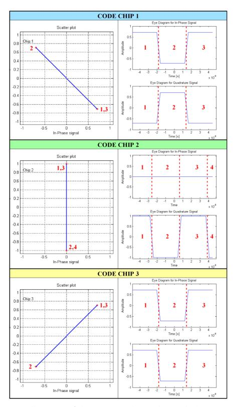
Figure 3.2: Illustration of the transitions during three code chips, caused by the subcarriers, in the scattering diagram and in the eye diagram of the AltBOC modulated signal
