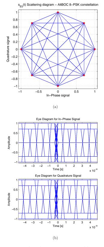
Figure 3.1: E5 AltBOC(15,10) scattering diagram (a) and eye diagram (b)
