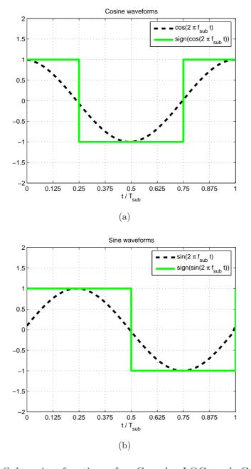
Figure 2.11: Subcarrier functions for Complex-LOC and Complex-BOC modulations: cosine waveforms (a) and sine waveforms (b)
