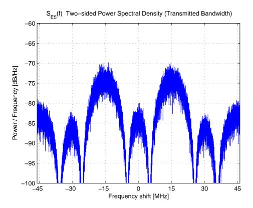
Figure 2.19: E5 AltBOC(15,10) signal spectrum
