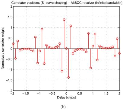
Figure 6.31: Correlator diagrams for infinite bandwidth receivers with the Scurve shaping technique: correlator positions and weights with the BPSK receiver in scenario 1 (a) and with the AltBOC receiver in scenario 2 (b)
