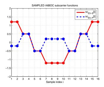
Figure 2.3: Sampled AltBOC subcarriers, with 16 samples per period
