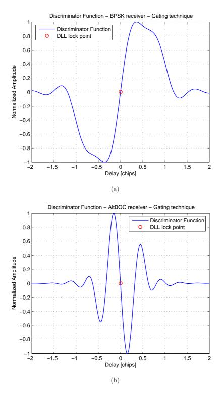
Figure 6.49: Discriminator functions obtained with the gating technique, for the two receiver architectures: discriminator function for the BPSK receiver (30 MHz) (a) and for the AltBOC receiver (51.150 MHz) (b)
