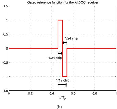
Figure 6.48: Gated reference functions for the gating technique, applied to the two receiver architectures: function for the BPSK receiver (a) and function for the AltBOC receiver (b)
