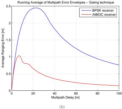
Figure 6.50: Multipath performances with the gating technique: multipath error envelopes (a) and running average of multipath error envelopes (b), for the two receiver architectures (BPSK receiver with 30 MHz and AltBOC receiver with 51.150 MHz)
