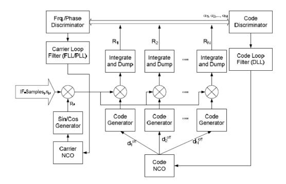
Figure 6.27: Generic multi-correlator channel architecture for the S-curve shaping technique [46]
