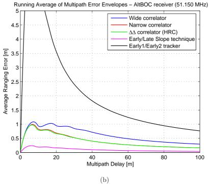
Figure 6.26: Comparison of multipath performances with the current mitigation techniques: running average of multipath error envelopes for the BPSK receiver (a) and for the AltBOC receiver (b)
