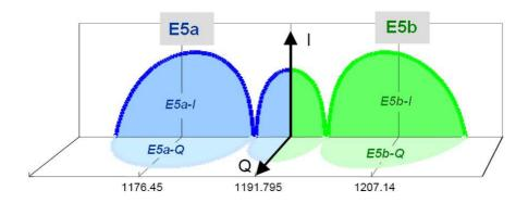
Figure 2.1: Spectral scheme for Galileo E5 band
