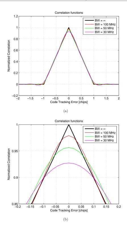
Figure 6.8: Comparison of the BPSK correlation peak, obtained processing only E5a for different signal bandwidths: shape of the correlation functions varying the bandwidth (a) and zoom around the correlation peak (b)
