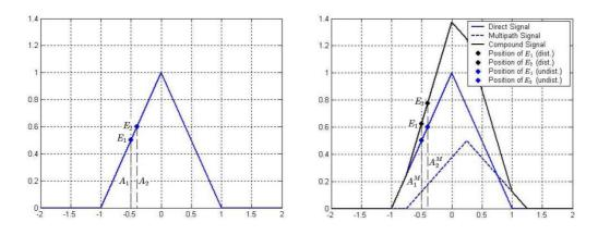
Figure 6.24: Basic  $E_1/E_2$  tracking concept [37]
