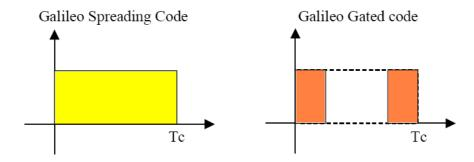
Figure 6.47: Galileo spreading code and its gated version [15]
