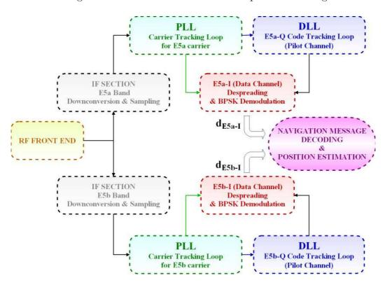
Figure 4.7: Block diagram of the separate dual band receiver architecture
