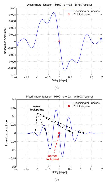
Figure 6.21: Discriminator functions with the High Resolution Correlator, using a spacing of d=0.1 chip, for the two receiver architectures: with the BPSK receiver (a) and with the AltBOC receiver (b)
