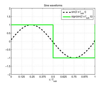
Figure 2.8: Subcarrier function for BOC modulation
