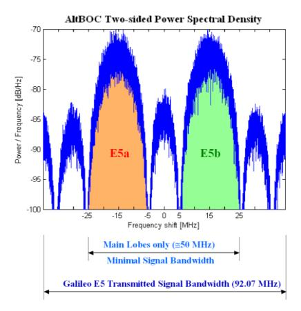
Figure 4.1: Galileo E5 AltBOC(15,10) signal bandwidth
