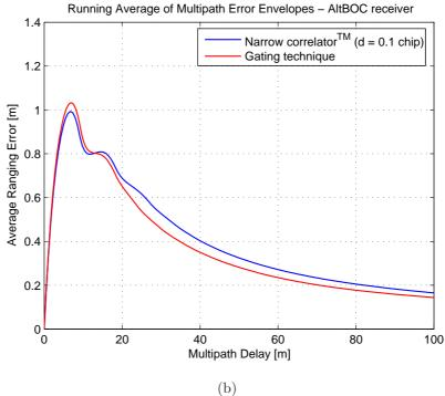
Figure 6.51: Comparison of multipath performances between the the narrow correlator  $^{\text{TM}}$  (with d = 0.1 chip) and the gating technique, applied to the two receiver architectures: the BPSK receiver (a) and the AltBOC receiver (b)
