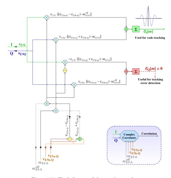
Figure 4.10: Block diagram of the complex correlator
