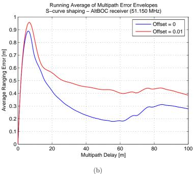
Figure 6.44: Comparison of multipath performances with the S-curve shaping technique, applied without offset or with offset: multipath error envelopes (a) and running average of multipath error envelopes (b) with the AltBOC receiver, using a bandwidth of 51.150 MHz and applying the S-curve shaping without offset (scenario 6) or with an offset of 0.01 (scenario 8)
