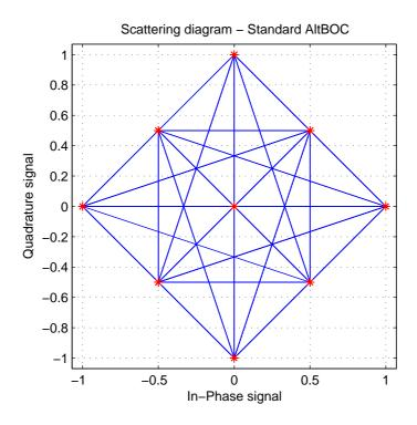
Figure 3.3: Standard AltBOC(15,10) scattering diagram
