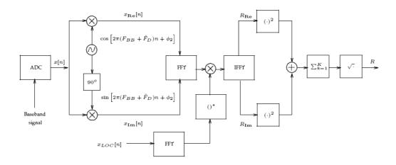
Figure 5.7: Non-coherent correlator implemented with a parallel search in the time delay domain [26]
