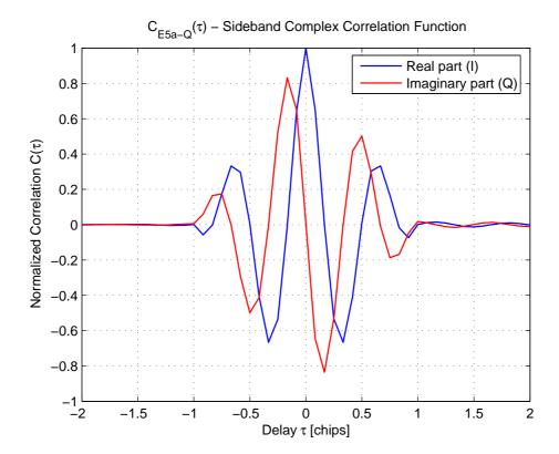
Figure 3.6: Sideband complex correlation function  $C_{E5a-Q}(\tau)$ , for the pilot channel of the E5a band
