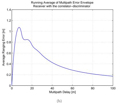
Figure 6.54: Multipath performances of the receiver with the correlatordiscriminator: multipath error envelopes (a) and running average of multipath error envelopes (b)
