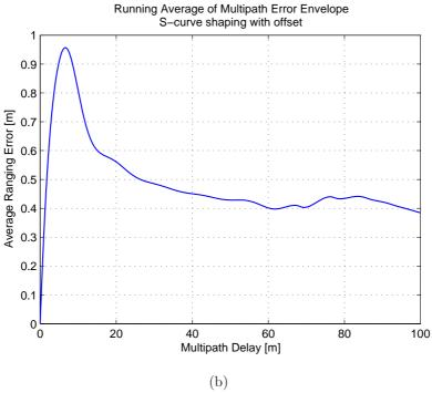
Figure 6.43: Multipath performances with the S-curve shaping technique with offset (scenario 8): multipath error envelope (a) and running average of multipath error envelope (b) with the AltBOC receiver, using a bandwidth of 51.150 MHz and an offset of 0.01 (normalized value)
