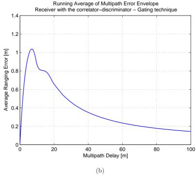
Figure 6.59: Multipath performances with the gating technique: multipath error envelopes (a) and running average of multipath error envelopes (b), for the receiver with the correlator-discriminator
