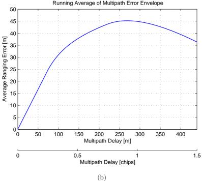
Figure 6.5: Examples of multipath error envelope (a) and running average of multipath error envelope (b), for the GPS C/A code ( $R_C = 1.023$  Mchip/s), considering an ideal receiver (infinite bandwidth) with a wide correlator (d = 1 chip)
