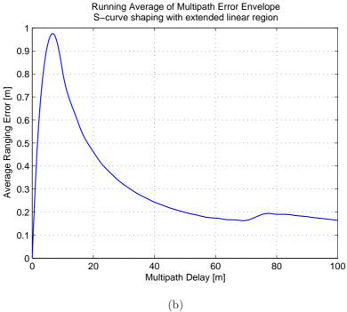
Figure 6.40: Multipath performances with the S-curve shaping technique with extended linear region (scenario 7): multipath error envelope (a) and running average of multipath error envelope (b) with the AltBOC receiver, using a bandwidth of 51.150 MHz and a linear region of  $\pm 2/12$  chip
