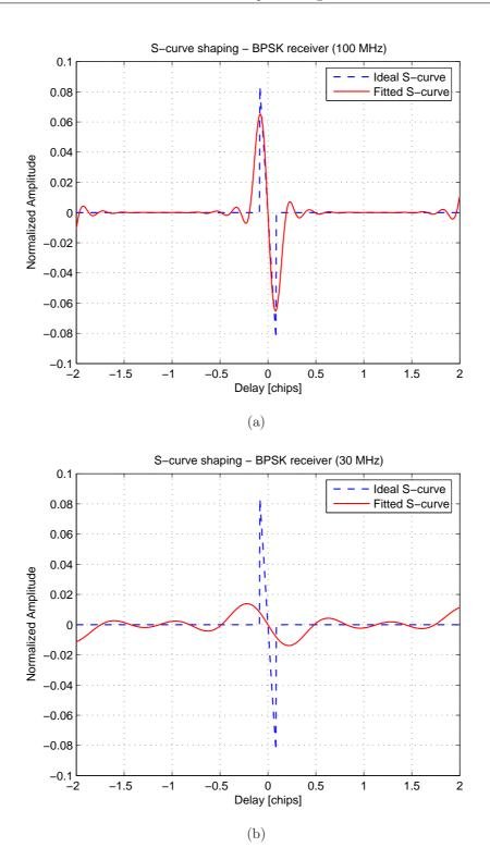
Figure 6.34: Ideal and fitted S-curves with the shaping technique, for the BPSK receiver with finite bandwidth signals: obtained S-curves in scenario 3 (a) and in scenario 4 (b)
