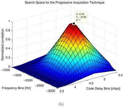
Figure 5.18: Example of SSB acquisition performed with the E5a-Q pilot code, simulated with a coherent dual band receiver in ideal conditions (with infinite bandwidth and without noise): resulting search spaces for the initial rough acquisition (a) and with the progressive acquisition technique (b)
