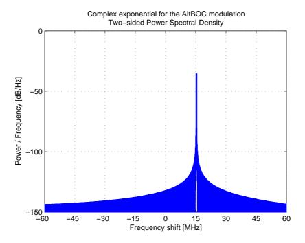
Figure 2.18: Spectrum of the complex exponential, used in the AltBOC modulation
