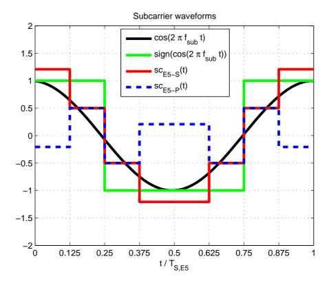
Figure 4.9: Different subcarrier functions for tracking options
