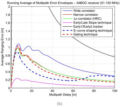
Figure 6.52: Comparison of multipath performances with current mitigation techniques and with emerging techniques: running average of multipath error envelopes for the BPSK receiver (a) and for the AltBOC receiver (b)
