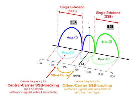
Figure 4.13: Different E5-band tracking options [8]
