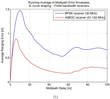
Figure 6.38: Comparison of multipath performances with the S-curve shaping technique, for the two receiver architectures using their respective optimal bandwidth (30 MHz and 51.150 MHz): multipath error envelopes (a) and running average of multipath error envelopes (b) with the BPSK receiver (scenario 4) and the AltBOC receiver (scenario 6)
