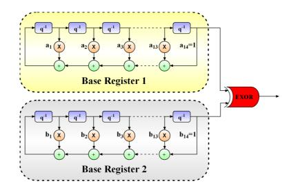
Figure 2.6: Primary code generation, with two shift registers
