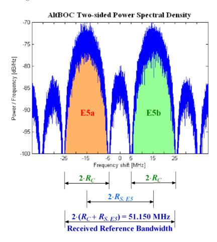
Figure 6.9: Illustration of the AltBOC received reference bandwidth
