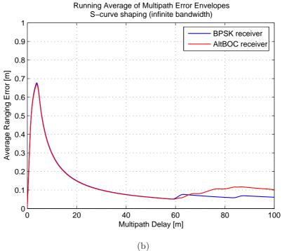
Figure 6.33: Multipath performances with the S-curve shaping technique, for infinite bandwidth receivers: multipath error envelopes (a) and running average of multipath error envelopes (b) for the BPSK receiver (scenario 1) and the AltBOC receiver (scenario 2)
