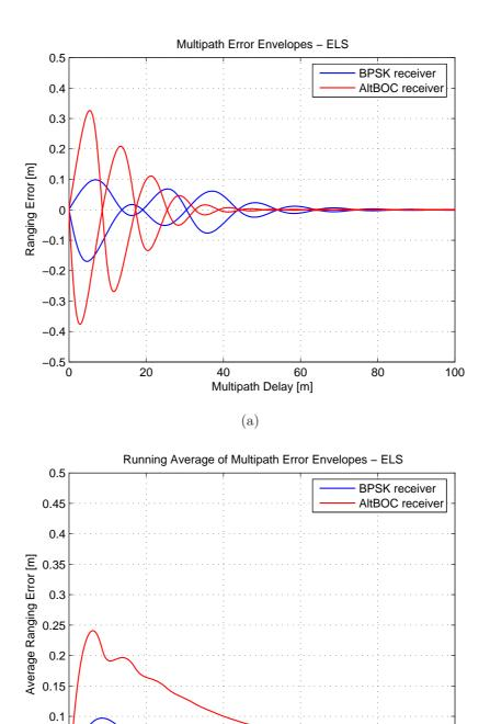
Figure 6.23: Multipath performances with the Early/Late Slope technique: multipath error envelopes (a) and running average of multipath error envelopes (b), for the two receiver architectures
