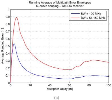
Figure 6.37: Multipath performances with the S-curve shaping technique, for the AltBOC receiver with finite bandwidth signals: multipath error envelopes (a) and running average of multipath error envelopes (b), for a bandwidth of 100 MHz (scenario 5) and 51.150 MHz (scenario 6)
