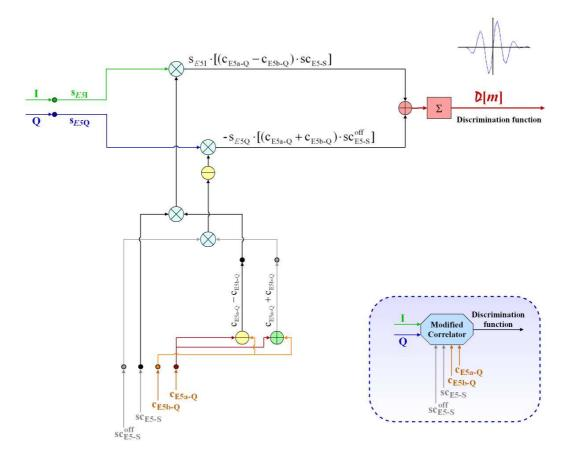
Figure 4.15: Block diagram of the correlator-discriminator
