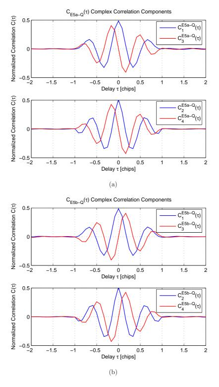
Figure 3.8: Components for the sideband complex correlation functions: in (a) the four components for  $C_{E5a-Q}(\tau)$ , and in (b) the four components for  $C_{E5b-Q}(\tau)$
