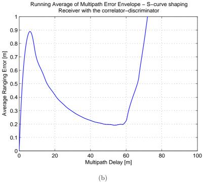
Figure 6.57: Multipath performances with the S-curve shaping technique: multipath error envelope (a) and running average of multipath error envelope (b), for the receiver with the correlator-discriminator
