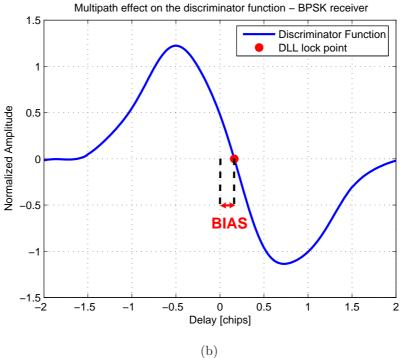
Figure 6.14: Multipath effect in BPSK receiver with wide correlator: alteration of the correlation function (a) and discriminator function distortion (b), assuming a reflected signal in phase with respect of the direct component, delayed by 0.5 chip and with  $\alpha=0.5$
