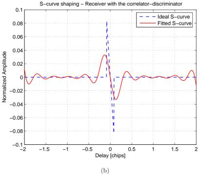
Figure 6.56: Correlator diagram and obtained S-curve with the shaping technique for the receiver with the correlator-discriminator: correlator positions and weights (a) and obtained S-curves (b)
