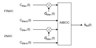
Figure 2.16: Modulation scheme for the E5 AltBOC signal [4]
