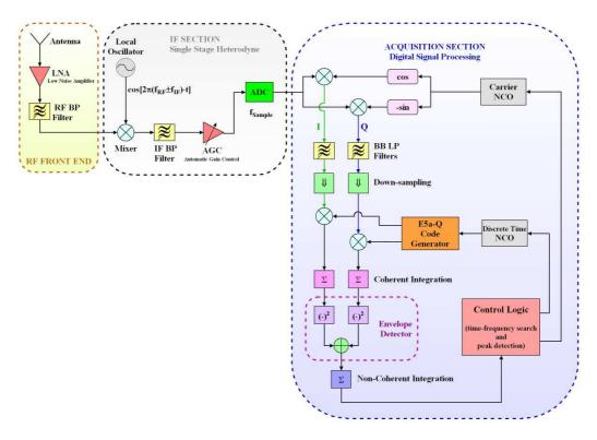
Figure 5.16: Block diagram of the coherent dual band receiver architecture, with the SSB (E5a sideband) acquisition section
