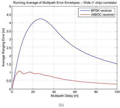
Figure 6.15: Multipath performances with the wide (standard) correlator: multipath error envelopes (a) and running average of multipath error envelopes (b), for the two receiver architectures
