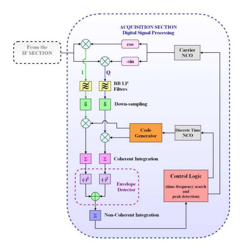
Figure 5.12: Block diagram of the acquisition section
