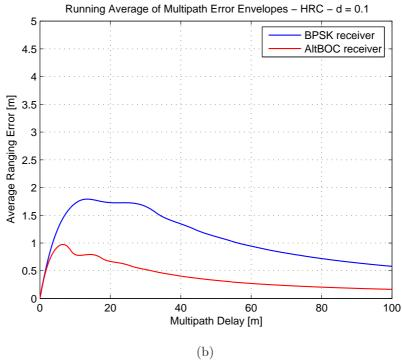
Figure 6.20: Multipath performances with the double delta correlator, using a spacing of d=0.1 chip: multipath error envelopes (a) and running average of multipath error envelopes (b), for the two receiver architectures
