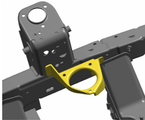
Fig. 4.1. Engine bracket: CAD model.
