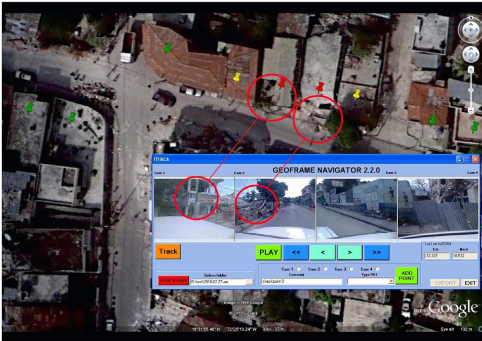
Figure 10. Comparison of a building damage classification on the aerial orthoimage and on the LCMMS frames – Erroneous classification example.
