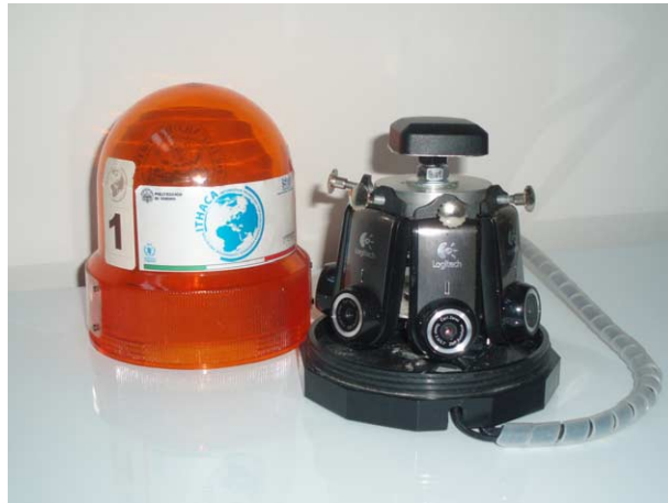
Figure 1. LCMMS system: four webcams and Global Positioning System (GPS) antenna embedded in a beacon light with a magnetic support.
