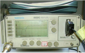
Fig. 1. Left: The frontal panel of the Tektronix 1502B reflectometer with rise time t_r = 0.3 ns. Right: A three arms probe.
