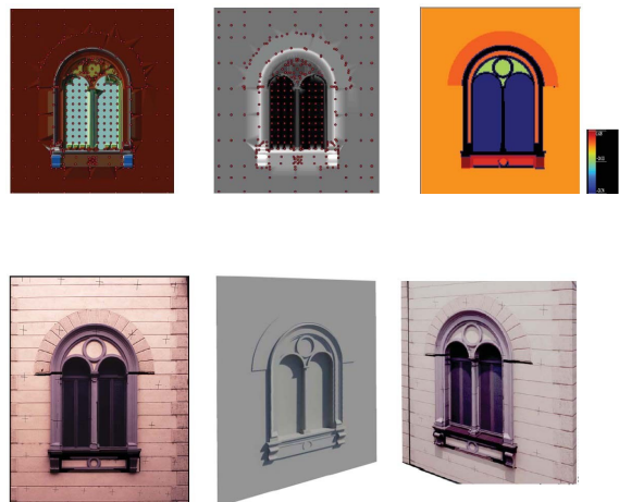
Figure 3: different level of details of documentation requirements demand different survey system. Continuous surfaces acquiring methods request suitable classification of elements strategies. In the picture sequence different processing phases (stereoplotting, dem processing, orthophoto and orthophoto 3D processing for a double lancet window). elaboration Presti.G.
