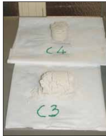
Figure 7. Example of two samples cured under natural soil and two cured in the open air. The difference in behaviour is clear.
