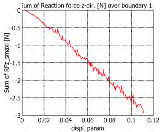
Figure 17. B-configuration: force exerted over the system vs displacement parameter ( displ\_param = 0.111 corresponds to appr\_dist = 0.141 mm).
