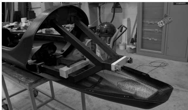
Fig. 15. Rear foam frame connected to the body.
