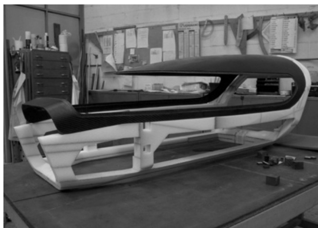
Fig. 12. Front foam frame (white colour).
