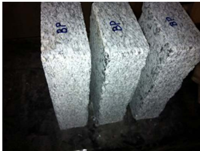
Figure 5. Adherence surface of stone treated by pneumatic drill
