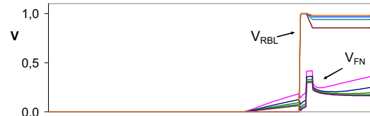
Figure 16 Incorrect readout of Q=0 due to O2 with resistance higher than 300\text{M}\Omega . The write and read actions are the same as in Figure 14.
