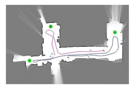
Figure 11: Map estimated through RBPF multi robot SLAM during experimental test at Politecnico di Torino. The corridor length is about 20 m whereas the particle set size was 100.
