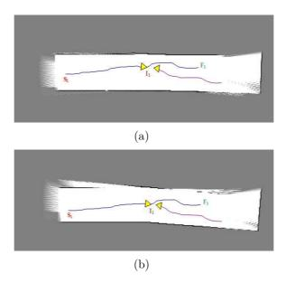
Figure 6: Toy example of multi robot RBPF-SLAM. In (a) the uncertainty in relative measurement is taken into account, whereas it is neglected in (b).
