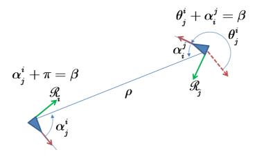
Figure 4: When a rendezvous event occurs each robot knows its final pose, respectively expressed in  $\mathcal{R}_{i0}$  and  $\mathcal{R}_{j0}$ , and is able to measure the relative pose of the teammate. It is possible to attach a reference frame to the rendezvous pose of each robot in order to understand how the overall transformation is the composition of the roto-translation between the represented reference frames.
