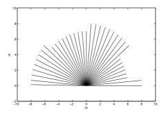
Figure 1: Range measurements from laser scanner at time t. The length of each radius is an entry of the vector  $z_{i,t}$ .
