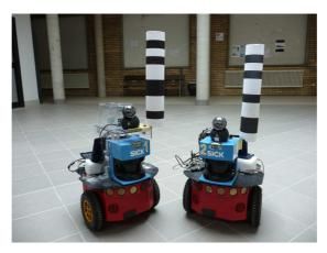
Figure 10: Robots P3-DX used for real tests. A bar code marker is used to distinguish the robots.
