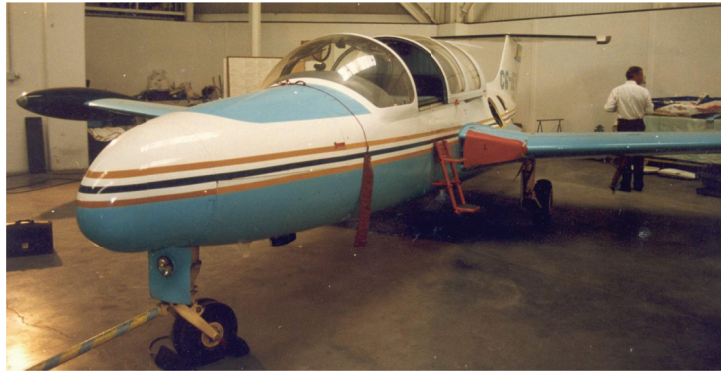
Figure 4: The plane twin to the crashed one. The aircraft was a double-jet executive plane, Morane Saulnier, 760 B model. Both the planes had been commissioned in November 1961.
