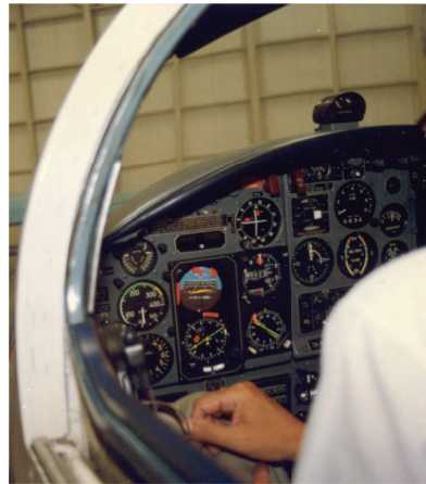
Figure 9: The triple indicator was positioned on the upper left corner of the airplane dashboard.
