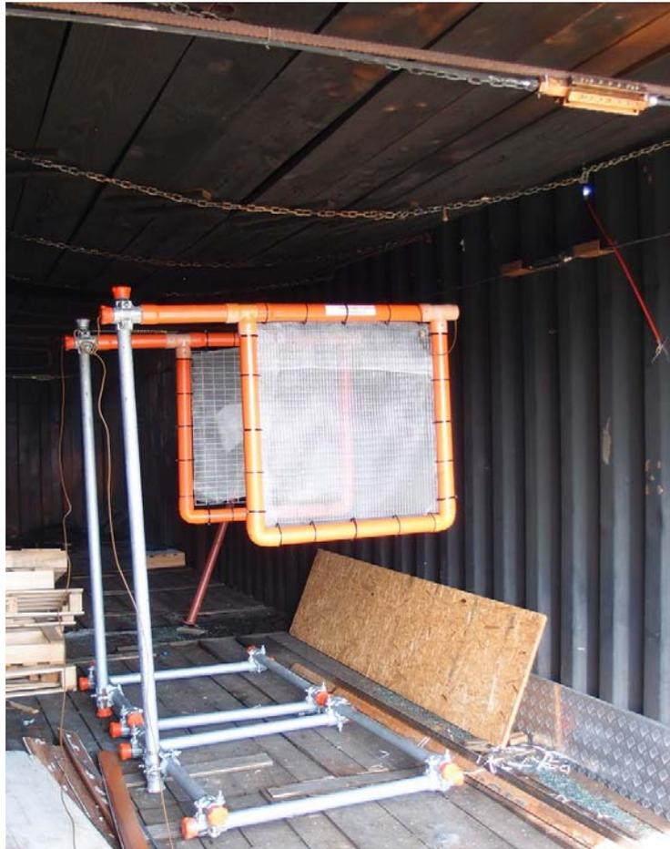
Figure 15. Targets used for wide fog measurements
