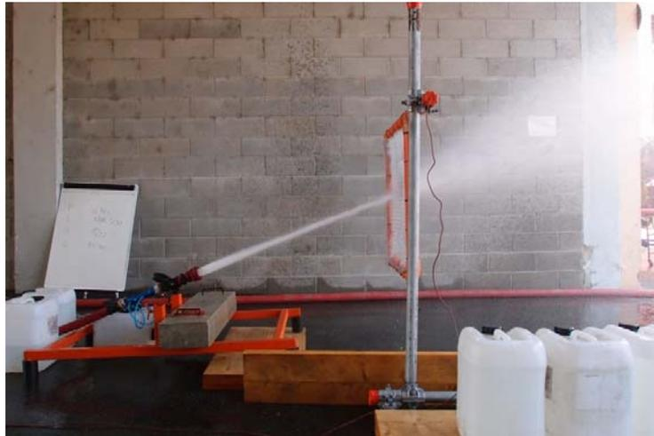
Figure 4. 'Pistol-grip' experimental set-up
