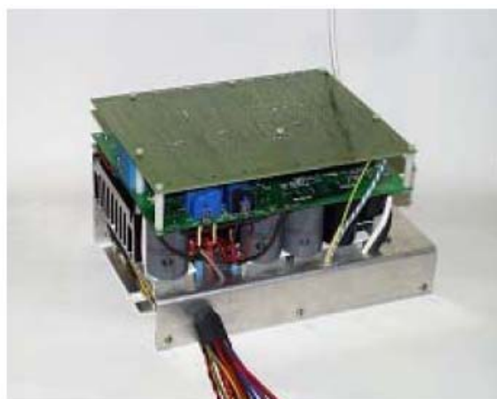
Fig. 5 – Converter for Big Electric Scooter.
