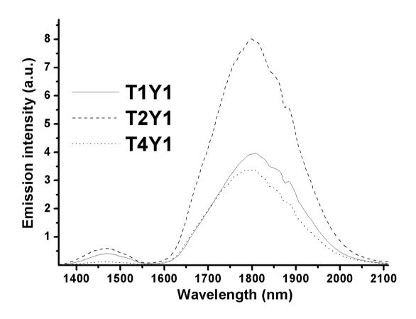
Fig. 6 – Fluorescence spectra of group III glasses (T1Yx glasses where  $x = mol\% Yb^{3+}$  ion), by pumping at 980nm.
