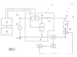
and emergency means 32 are activated when the monitored parameter value exceeds the respective reference value. The electric parameter may be the current flowing through the piezoelectric actuator 19 and/or the low-side driver 21, sensed by current sensor 30, or the voltage across the piezoelectric actuator. The emergency means 32 may interrupt the operation of the drivers 20, 21, discharge the piezoelectric injector or disconnect the injector form the power circuit 17.
