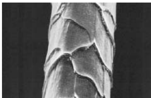
Figure 12.1 A wool fiber in covered by cuticle scales. Very long cells are building the inner structure of the fiber.
