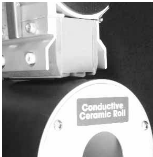
Figure 9.2 A treatment station with a conductive ceramic roll
