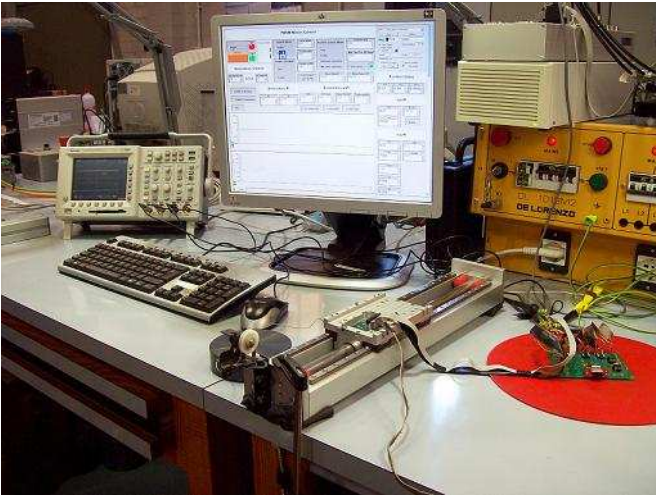
Figure 10. LPMSM prototype used for the tests.
