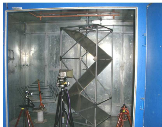
Figure 1: AARC prototype. Inside: the “Z-fold” stirrer, a logperiodic excitation antenna, a conical dipole receiving antenna, the field probe and a dummy EUT.
