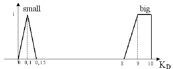
Fig. 12. Membership functions of the output variable K_D
