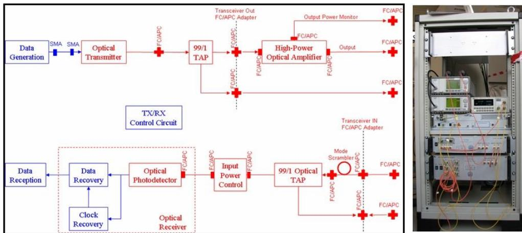
Fig. 6. Transceiver design.
