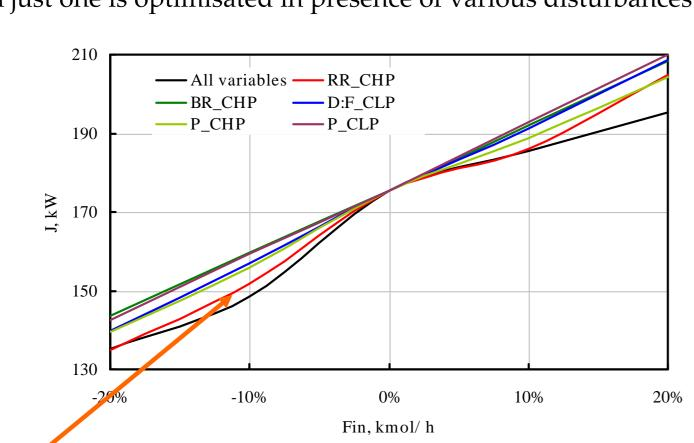
The optimisation of the reflux ratio of the high pressure column is enough to fulfill the constraints and to minimise the cost function
