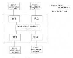
Fig. 6. Distributed Setup. Star Topology
