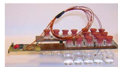
Figure 2. Load cell and wireless thermometer.
