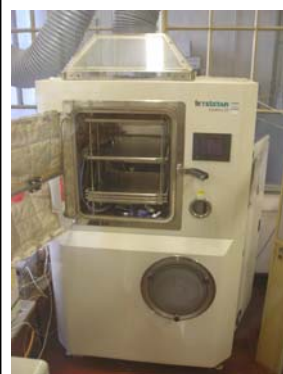
Figure 7. The pilot freeze-dryer used for experiments
