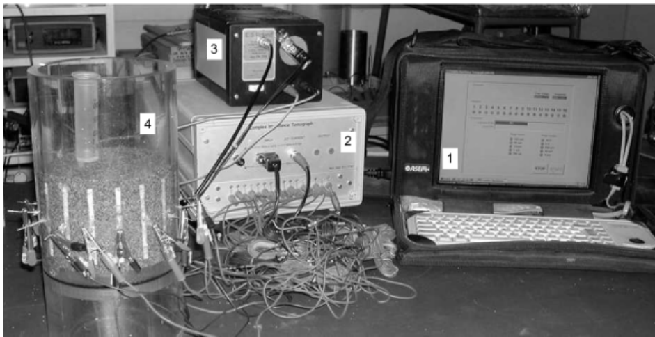
Fig. 1. Measurement set-up: 1, personal computer; 2, data acquisition system; 3, inverter; 4, measuring cell
