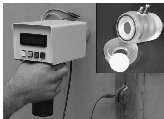
Fig. 2. System during an outside measurement of a common painted metallic door and a detailed photo of the electrochemical cell.
