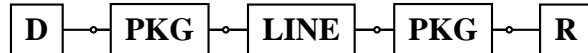
Figure 1: Main parts of a generic board-level interconnected system. D : drivers; PKG : packages; LINE : interconnect; R receivers.
