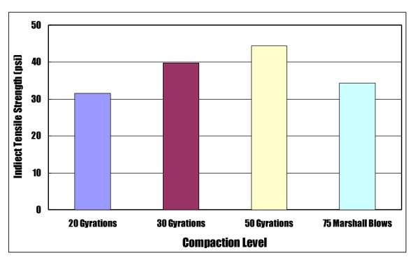
Figure 6-3. Comparison of average indirect tensile strength at four different compaction levels
