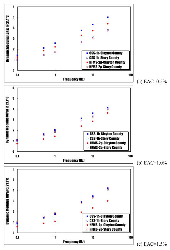
Figure 8-4. Plots of dynamic moduli against six loading frequencies for three emulsified asphalt contents at  $21.1^{\circ}$ C
