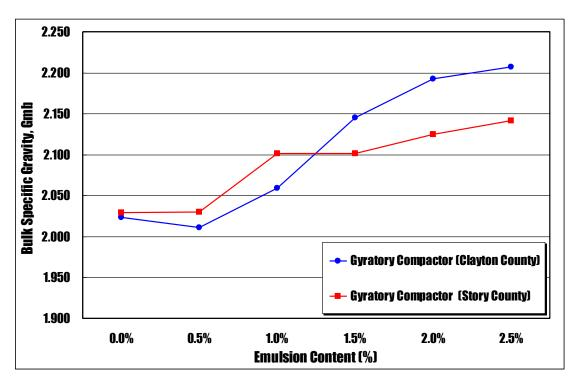
Figure 7-1. Plots of bulk specific gravity against emulsified asphalt content for gyratory compacted CIR-CSS-1h specimens using different RAP materials
