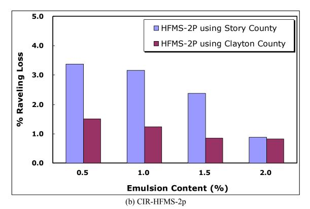
Figure 8-24. Percent raveling losses for two different CIR-emulsion specimens from two different RAP sources
