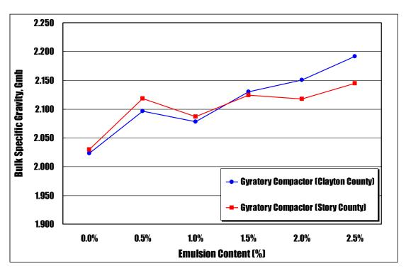
Figure 7-3. Plots of bulk specific gravity against emulsified asphalt content for gyratory compacted CIR-HEMS-2p specimens using different RAP materials
