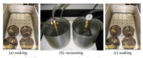
Figure 7-10. Vacuum saturation procedure for making wet specimens
