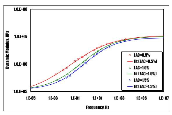
Figure 8-8. Mater curves for CIR-HFMS-2p from Clayton County at three EACs
