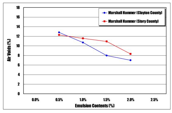
Figure 7-7. Plots of air void against emulsified asphalt content for Marshall compacted CIR-CSS-1h specimens using two different RAP materials
