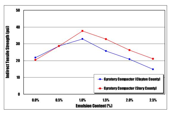
Figure 7-11. Plots of indirect tensile strength against emulsified asphalt content for Gyratory compacted CIR-CSS-1 specimens using two different RAP materials
