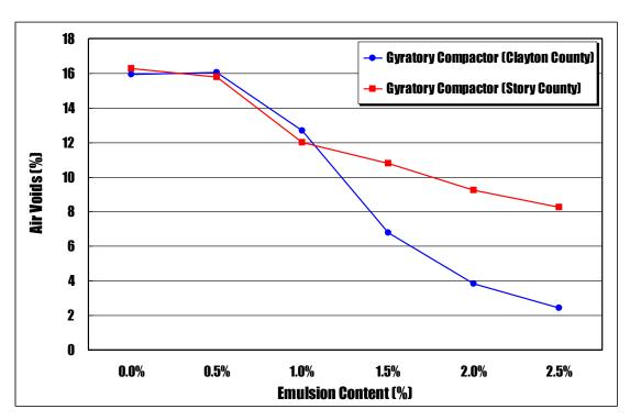
Figure 7-6. Plots of air void against emulsified asphalt content for gyratory compacted CIR-CSS-1h specimens using two different RAP materials
