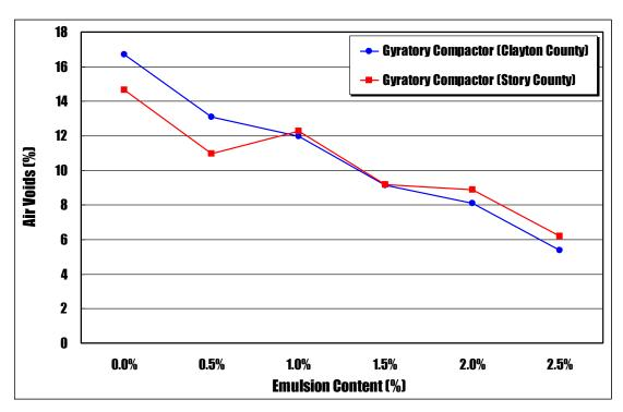
Figure 7-8. Plots of air void against emulsified asphalt content for gyratory compacted CIR-HFMS-2p specimens using two different RAP materials
