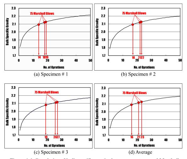
Figure 6-4. Correlation of bulk specific gravity between gyratory and Marshall compacted CIR-CSS-1h specimens
