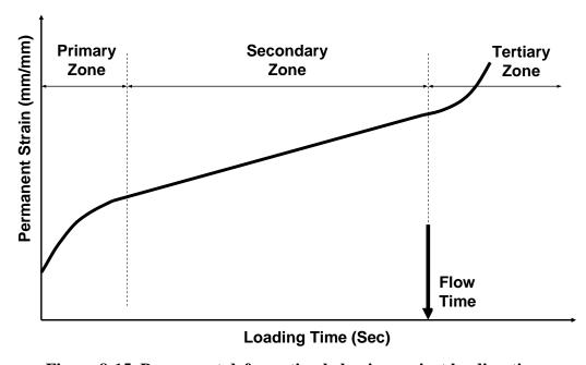
Figure 8-15. Permanent deformation behavior against loading time
