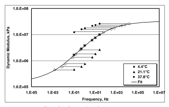
Figure 8-1. Construction of master curve
