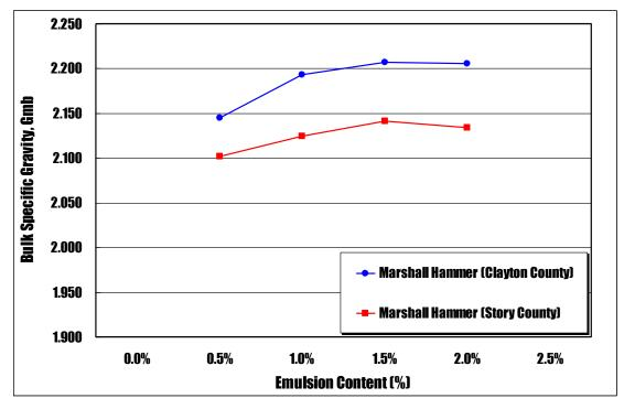
Figure 7-4. Plots of bulk specific gravity against emulsified asphalt content for Marshall compacted CIR-HFMS-2p specimens using different RAP materials
