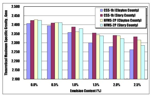
Figure 7-5. Bar charts of theoretical maximum specific gravities against emulsified asphalt content for two emulsion types and two RAP sources
