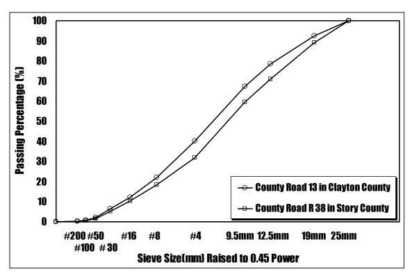
Figure 5-3. Gradation plots of two RAP materials passing 25mm sieve
