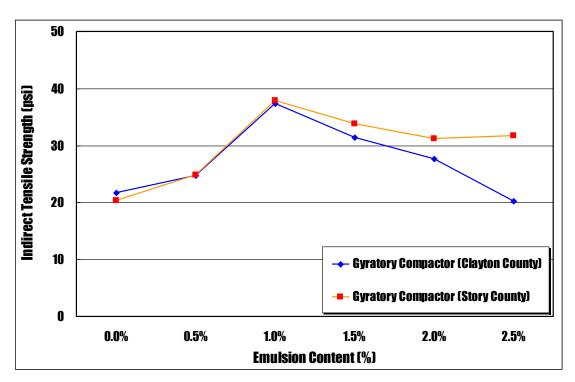
Figure 7-13. Plots of indirect tensile strength against emulsified asphalt content for gyratory compacted CIR- HFMS-2p specimens using two different RAP materials
