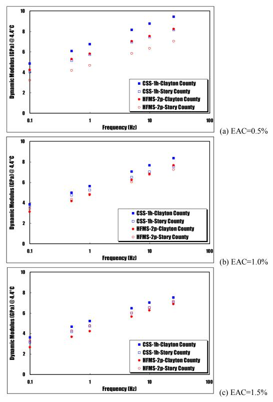
Figure 8-3. Plots of dynamic moduli against six loading frequencies for three emulsified asphalt contents at 4.4°C
