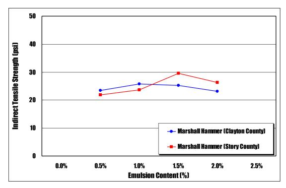
Figure 7-12. Plots of indirect tensile strength against emulsified asphalt content for Marshall compacted CIR-CSS-1 specimens using two different RAP materials
