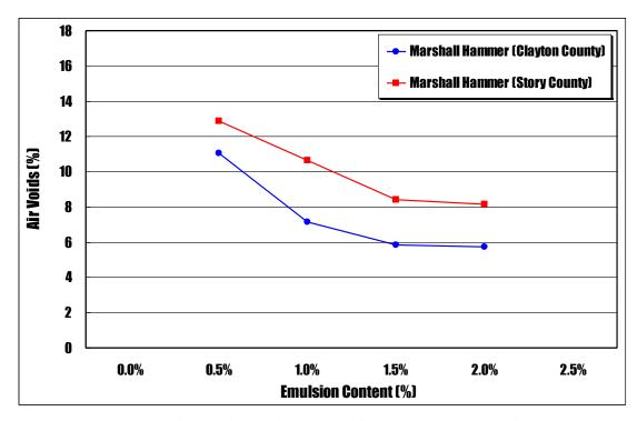
Figure 7-9. Plots of air void against emulsified asphalt content for Marshall compacted HFMS-2p specimens using two different RAP materials
