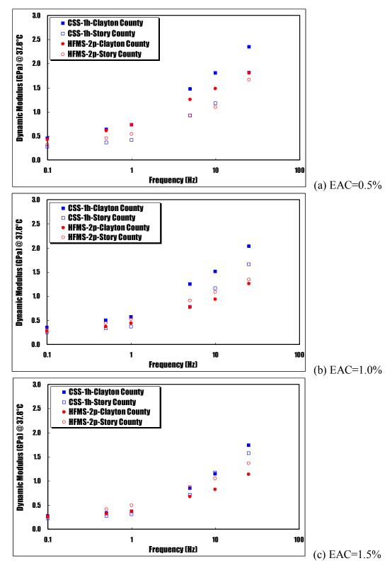
Figure 8-5. Plots of dynamic modulus value against six loading frequencies for three emulsified asphalt contents at 37.8°C
