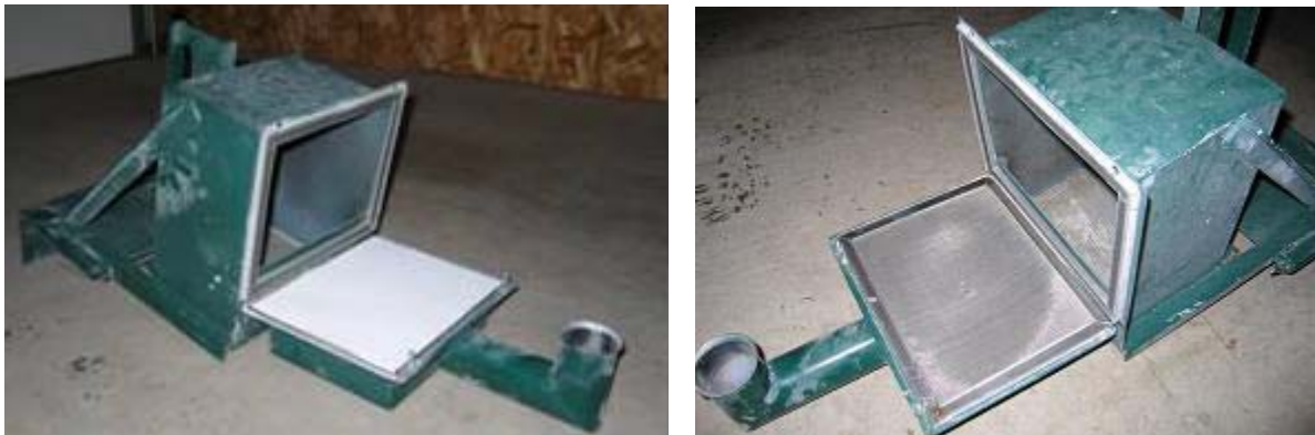
Figure 5.1.5. Opened filter box with and without filter paper.
