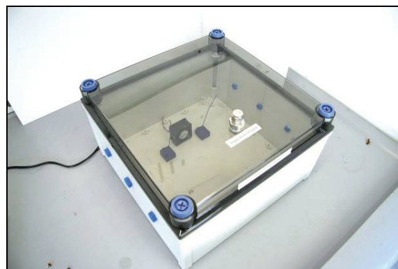
Fig. 3 – The low volume environmental testing chamber
