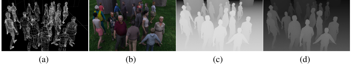
Figure 4.20: Synthetic data generation; (a) 3D model wireframes; (b) Rendered scene; (c) Groundtruth depth map; (d) Groundtruth disparity map.
