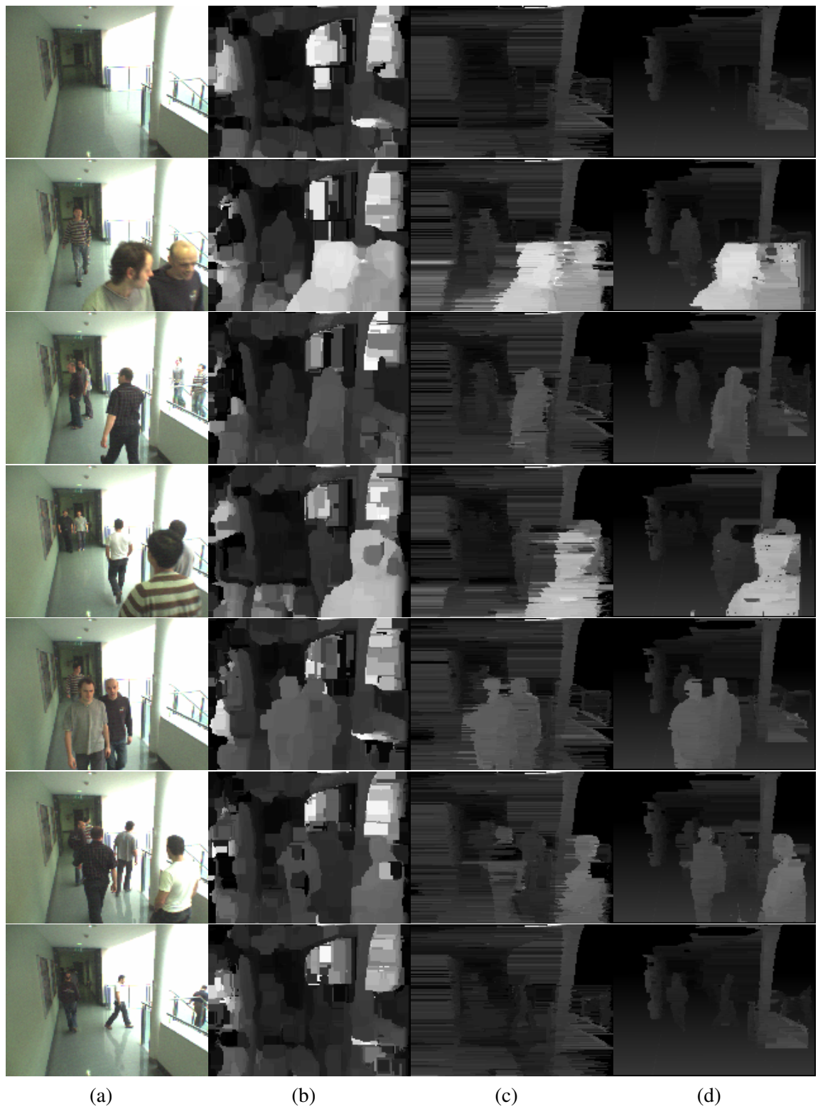
Figure 4.28: Corridor scene results; (a) Input; (b) SSD_{sw35\_t1000} ; (c) SSD_{DP\_o400\_s400\_t1000} ; (d) Proposed approach.
