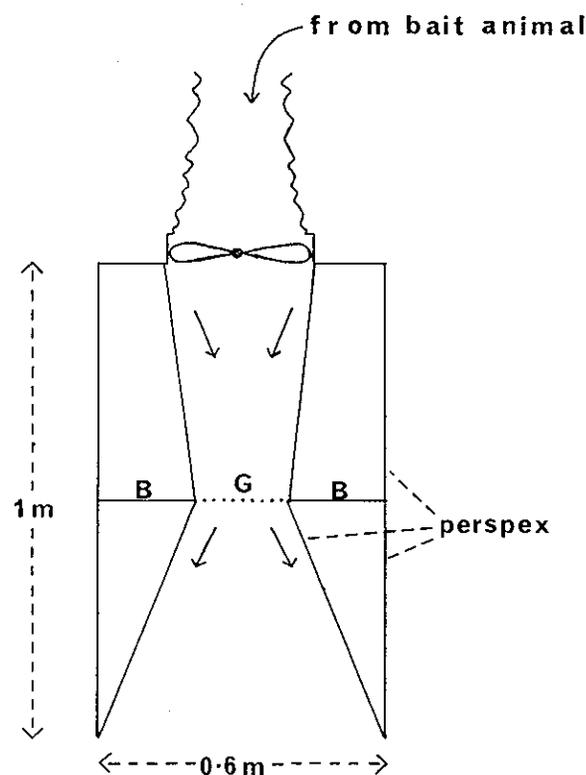
Fig. 2.—Plan view of wind tunnel. (*G*, electrocuting grid; *B*, transverse baffle.)
