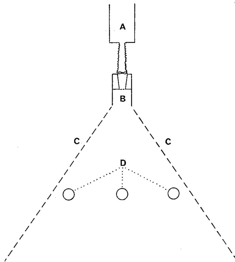
Fig. 1.—Plan of experimental field wind tunnel. (*A*, animal stall; *B*, wind tunnel; *C*, 1-m high fence; *D*, suction traps.)
