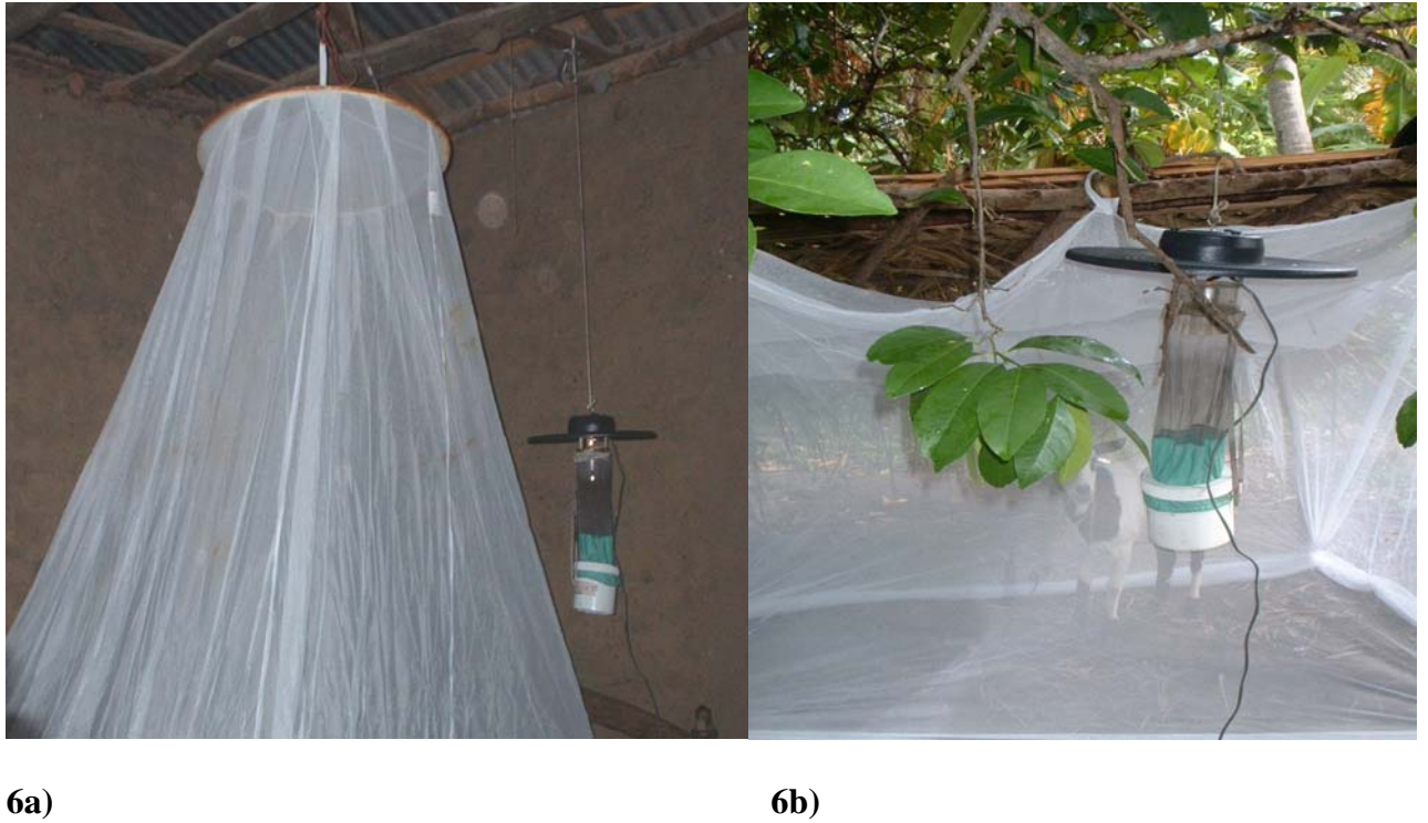
Figure 6: 6a. Set up of human baited trap with CDC light traps; 6b. Set up of animal baited trap with CDC light trap.
