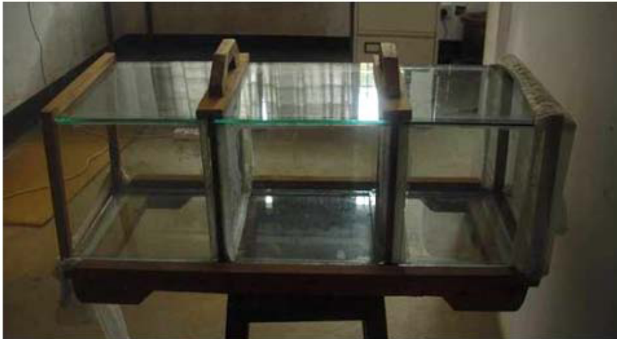
Figure 1 Behavioural chamber with three equally sized compartments: release, middle, and stimulus compartment. A guinea pig (Experiment 1) or a worn sock (Experiment 2) was placed in the stimulus compartment.
