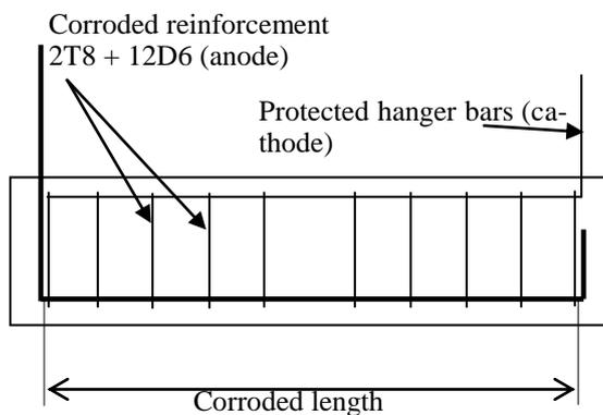
Figure 1. Beam specimens.
