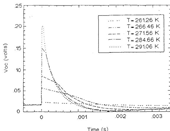
Fig. 5.  $V_{oc}$  decay curves for an a-Si:H p-i-n cell following light soaking.
