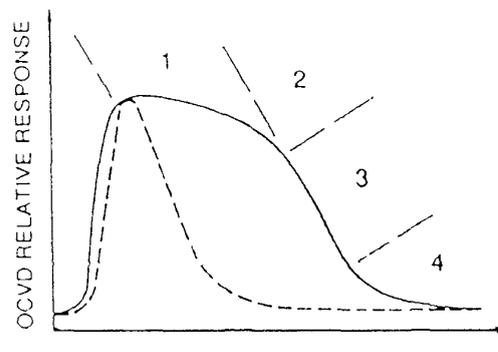
Fig. 1. A comparison of a typical OCVD response for an amorphous silicon module to the excitation pulse showing the four decay modes: 1, intrinsic; 2, trap activation; 3, trap-assisted intrinsic decay; 4, final non-linear exponential decay.
