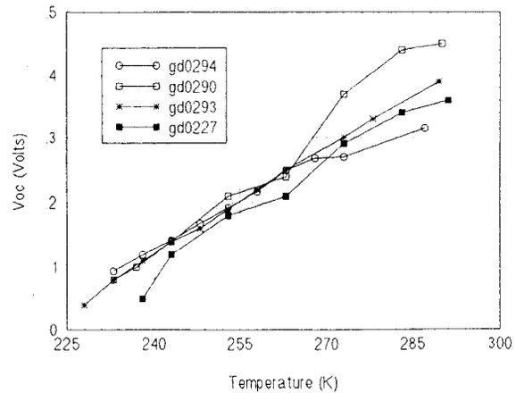
Fig. 4. V<sub>oc</sub> vs. temperature for a-Si:H, p-i-n cells.
