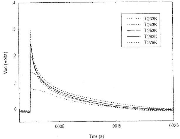
Fig. 3. V<sub>oc</sub> decay curves for an a-Si:H p-i-n cell at various temperatures.
