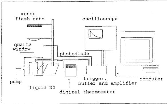
Fig. 2. Experimental arrangement for the measurement of the open-circuit-voltage-decay
