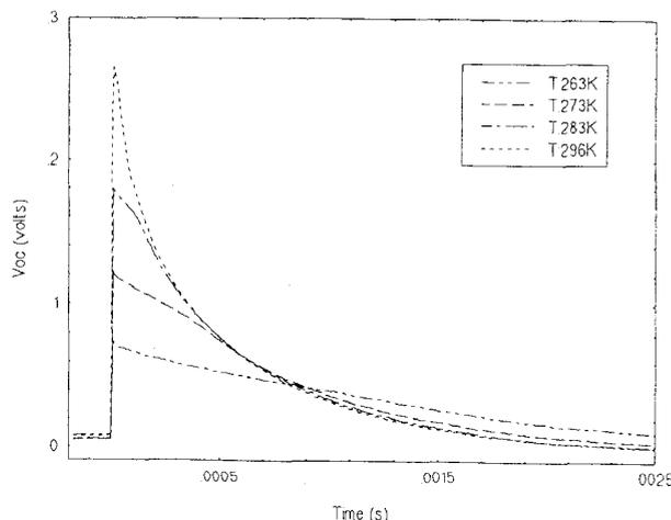
Fig. 6.  $V_{oc}$  decay curves for an a-Si:H, p-i-n cell after exposure to AM1 illumination.
