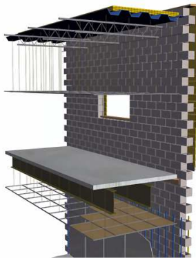
FIGURE 7 ABOVE-CEILING COMPONENTS (ACC) MODEL
